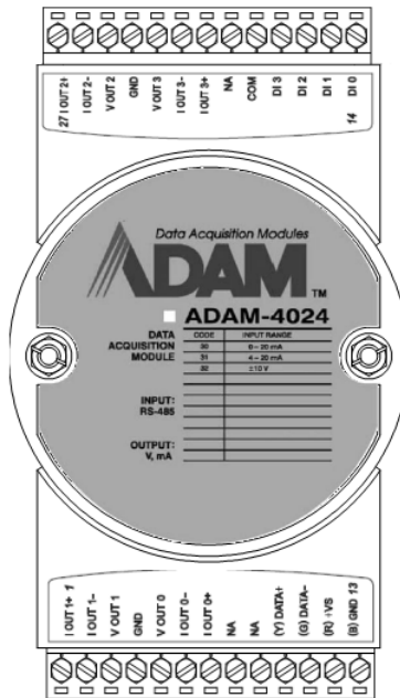
Figure 3-38 ADAM-4024 4-channel Analog Output Module
