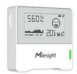
AM103 is a 3-in-1 ambience monitoring sensor including the measurement of temperature, humidity and CO<sub>2</sub> concentration and can display indoor status visually on the E-ink screen in real-time and transmit to network server using LoRaWAN® technology.
