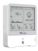
AM319 is a 9-in-1 ambience monitoring sensor including the measurement of temperature, humidity, CO<sub>2</sub> concentration, TVOC, pressure, light, motion, PM2.5 & PM10, HCHO/O<sub>3</sub>, etc. It can show visually with differ modes on the E-ink screen in real-time and transmit to network server using LoRaWAN® technology.
