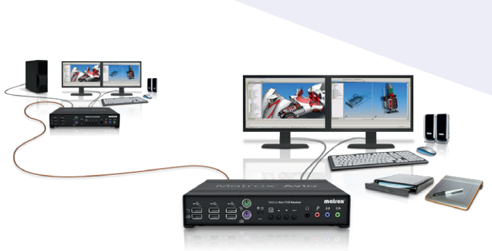
Matrox Avio F125 extends dual-digital video and USB 2.0 devices by up to 10 km (6.2 mi) over a single fiber-optic cable.
